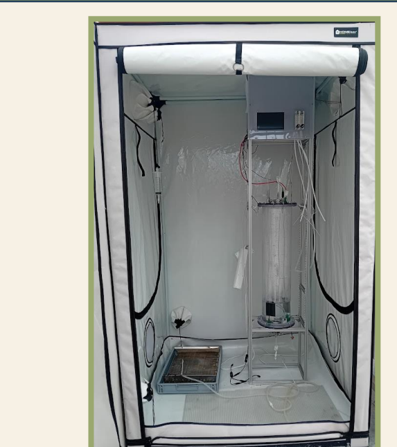
Closed reactor tube (25 L) in a growth tent setup
